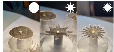
Fig. 1 Various designs of evaporator in solar desalination system
